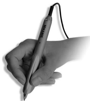
Figure 1: Signature acquisition device
